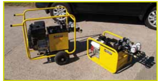
Petrol powerpacks for re-railing applications.
