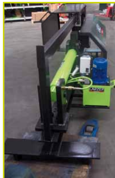
Wheel crusher. 23Tn capacity and 800 mm stroke.
