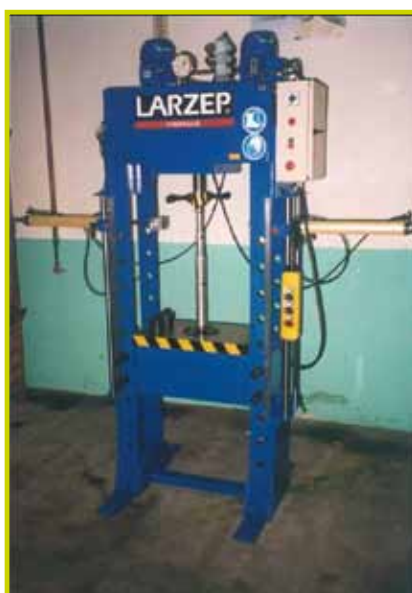
Precision press for production purposes with safety systems.
