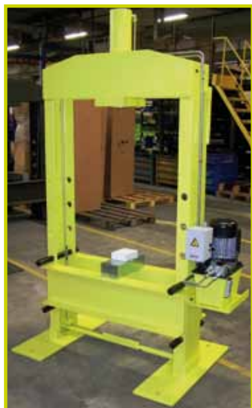
Double acting 50 Tn capacity and 370 mm stroke press with powerpack.
