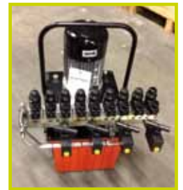
Powerpack with solenoid valve and by-pass, to work with 4 cylinders independently.
