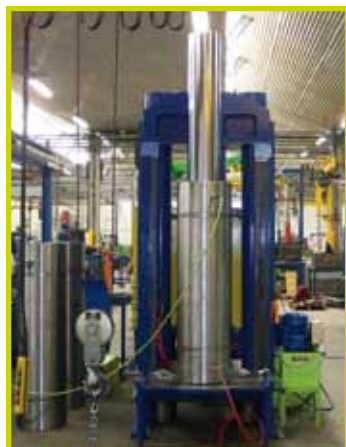
Double acting cylinder with 1.250 mm stroke.
