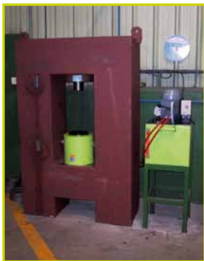
30 Tn capacity and 90 mm stroke press with 50 litres powerpack with 4 ways.
