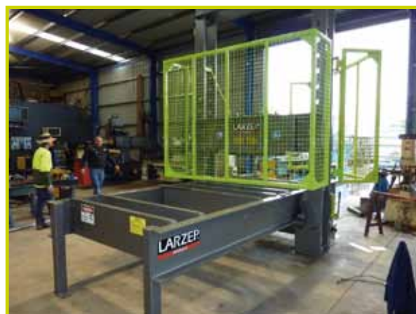
Moving column press, 200 Tn capacity.
